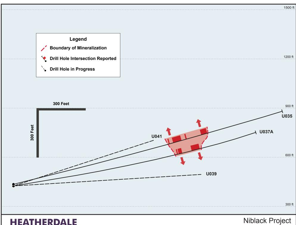
Drill Station 2 - Vertical Cross Section Looking Southeast
