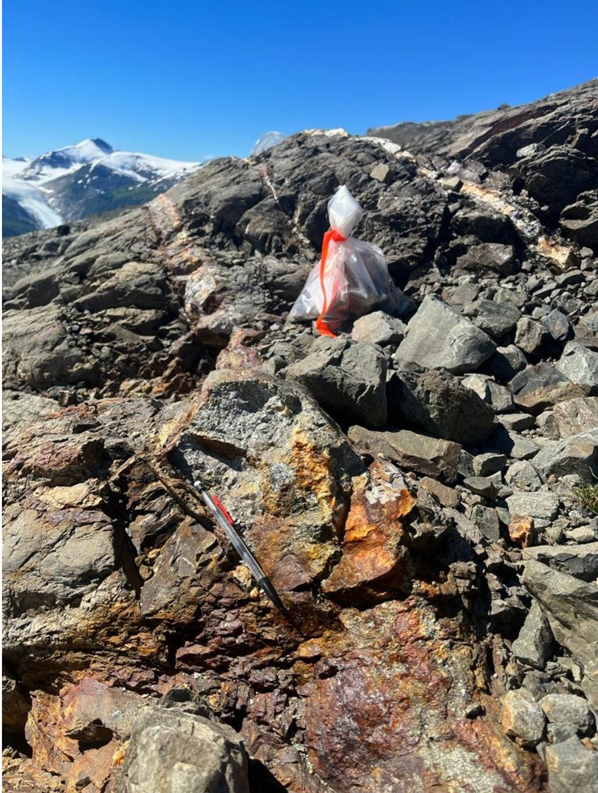
Figure 5 – Quartz-sulfide veining at Doghole Prospect, Texas Creek Property. Location of sample B0010766: 16.6 g/t Au and 585 g/t Ag
